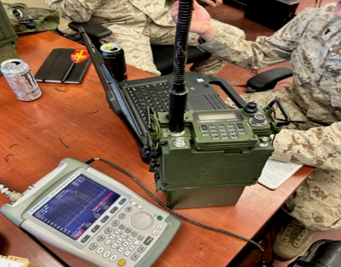
ECC Marines learning what different radios waveforms look like on different power setting using spectrum analyzer.
